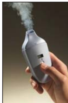
Figure 2. Chrysalis Technologies' Aria™ (Functional prototype) portable inhaler for pulmonary drug delivery.
