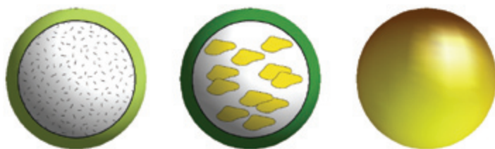
Figure 1. Schematic drawing of microcapsules and microspheres. From left to right: Microcapsule with solution as core, microcapsule with cell suspension as core, and microsphere with matrix-encapsulated active agent.
