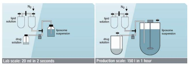
Figure 1. Production of liposomes at different scales.
