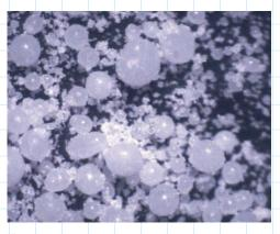
Figure 1. Stereomicroscope image of MCP-CeCo50 VarioSol® microparticles.
