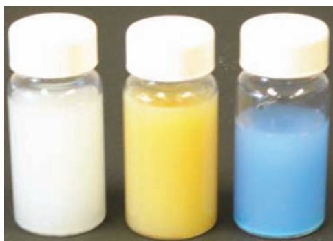
Figure 1. Self-assembly of peptides with encapsulated (left to right) \text{Ca}^{2+} , \text{Fe}^{3+} , and \text{Cu}^{2+} .
