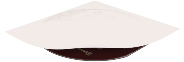
Film is peeled off of silicon wafer using water soluble tape
