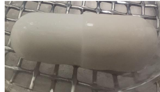
Exemplar image of custom enteric capsule filled with C8 after 2h in HCl 0.1N (no sinker, no disk)
