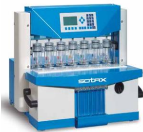
Figure 6: Continuous flow method and flow through dissolution system
