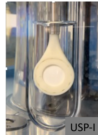
3D-Printed Two-side Adapter in USP apparatus I
