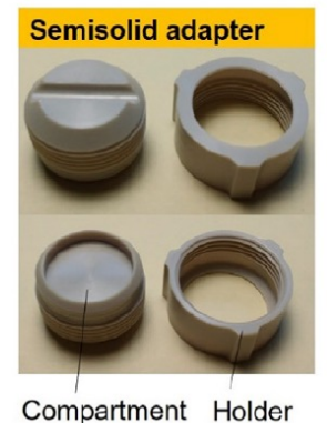
C: USP apparatus 4 with semisolid adapters
