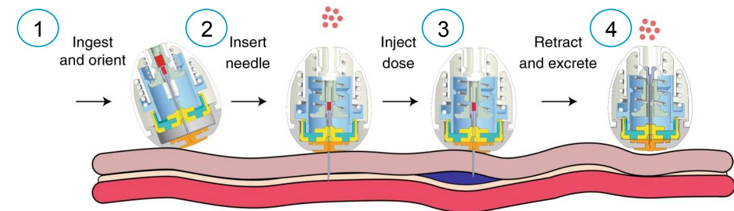
Staged and sequence controlled multi-spring actuation system that injects a hypodermic needle beneath the gastric mucosa and, thereupon, delivers 80  $\mu$ l of liquid drug formulation into the submucosal space.
