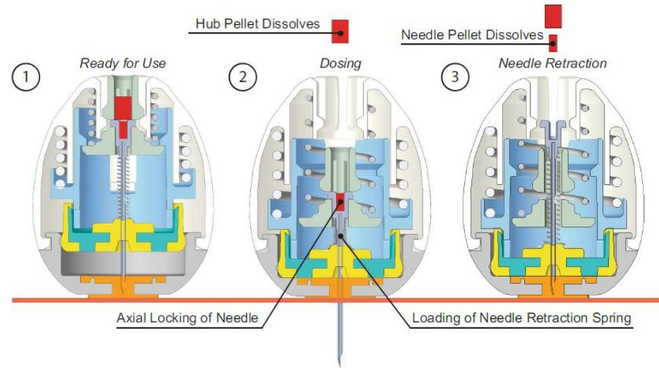
The device first actuates after the hub pellet (red) dissolves and allows the latching mechanism at the top of the pill to release. The retraction spring, located axially around the needle shaft, compresses after the first stage of actuation due to the inherent movement of the needle during injection. The dissolution of the second pellet, which is exposed only after the first pellet dissolves, frees the spring to expand and draw the needle back into the capsule.
