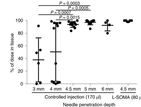
Percent of contrast dye that remained in tissue after injection calculated using 3D reconstructions of MicroCT images
