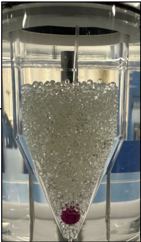
22.6 mm Compendial Cell, Implant vertically seated in beads
