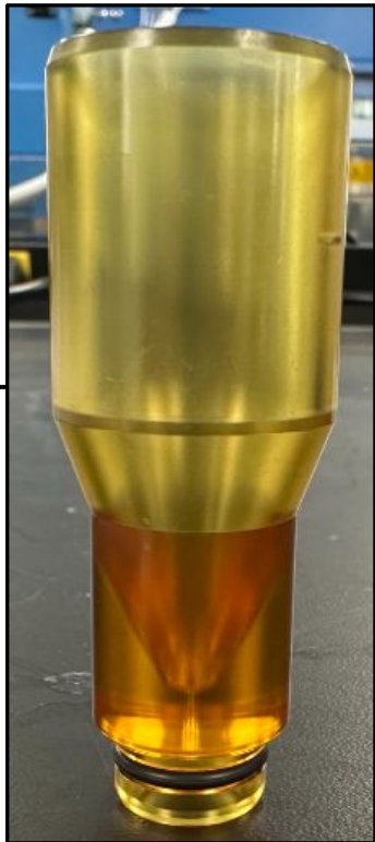
22.6 mm Compendial Cell Utem cell, more chemically resistant material
