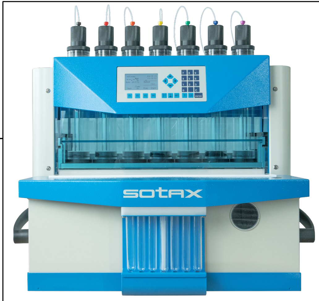
Base CE7 was modified to be able to fit Large Stents
